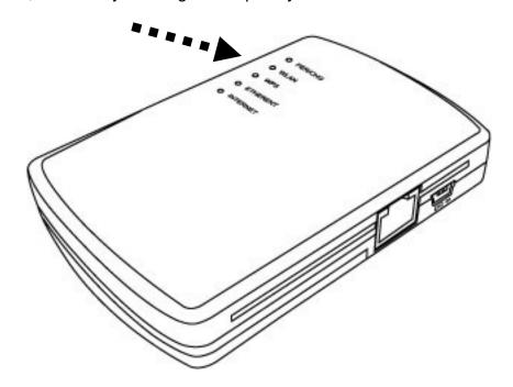
Note: The 'Power' LED is lit in green color when the battery is charged completely if router is activated before charged.
